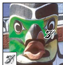
The History Brush tool paints a copy of the selected state or snapshot into the current image window.
