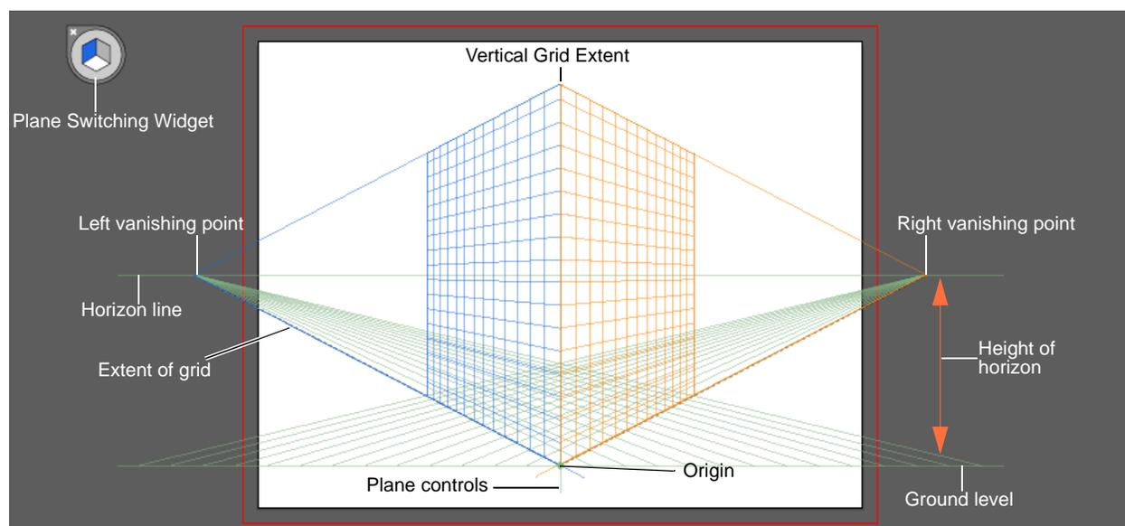
**Figure 1** Perspective grid illustrating two-point perspective
