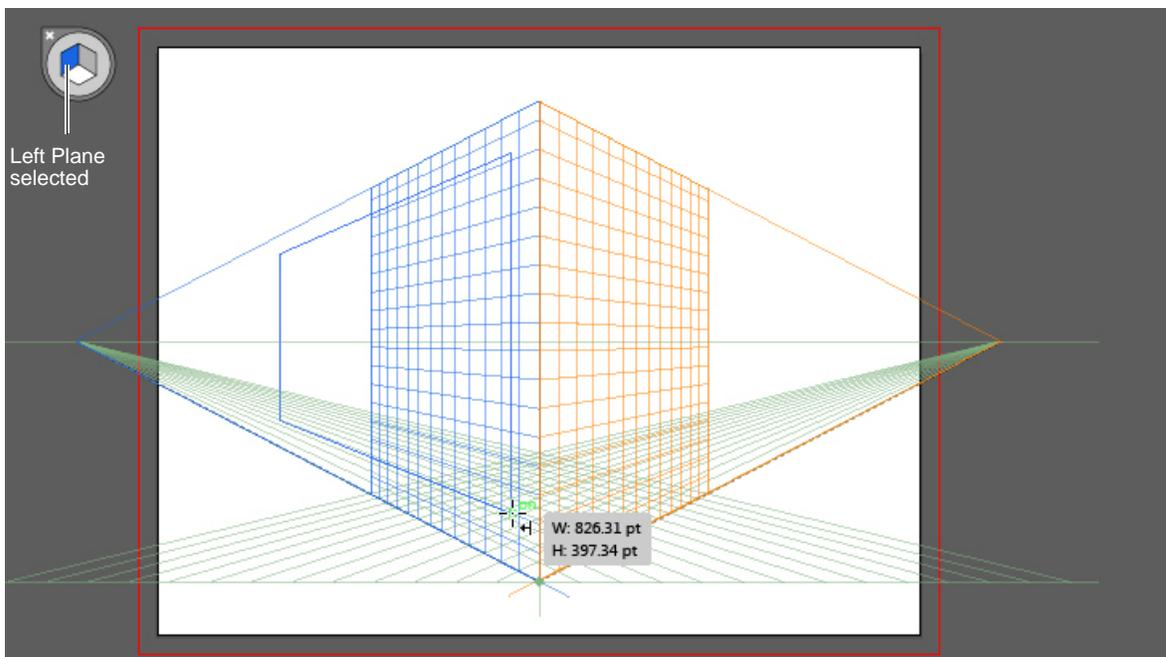
**Figure 6** Drawing a rectangle in the perspective grid
